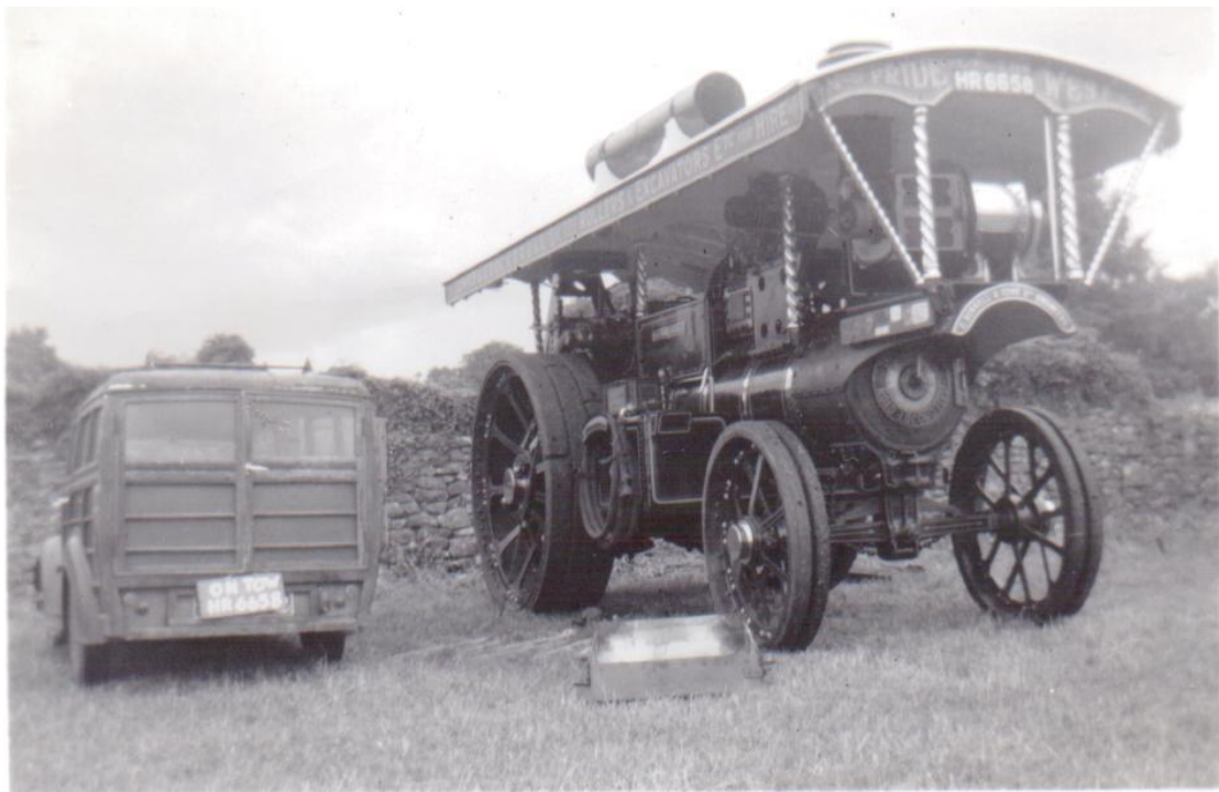
The Prince of Wales (1922 Burrell 3887) at Nunney Fete, note the ash pan and fire bars removed to access the leaking boiler tubes in the fire box.
